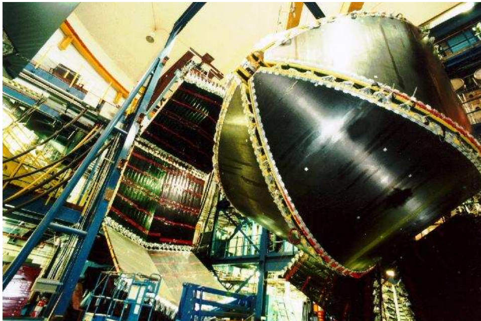
Figure 2.8: Photograph of the CLAS detector taken during a maintenance period for which the time-of-flight scintillator walls, forward region Cerenkov counters and electromagnetic calorimeters were pulled away from the interior detector elements. Image Source: [33].
