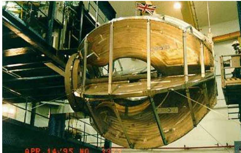
Figure 2.9: The CLAS magnet separated from the rest of the detector before installation [18].
