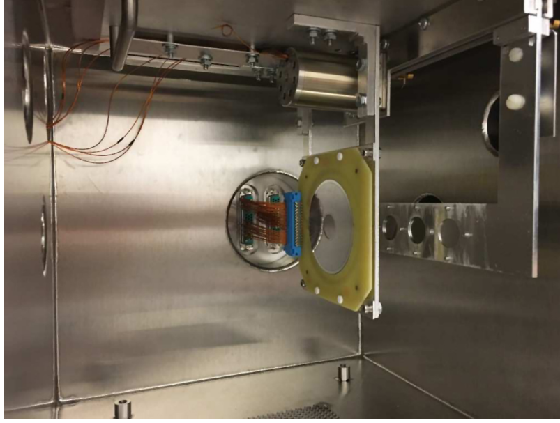
Figure 2.9: Picture of the TPOL detector inside the vacuum enclosure. The beam enters from the right, passes through the beryllium foil mounted on the L-shaped beam, and proceeds into the experimental hall. The SSD is mounted after the beryllium foil. Reproduced from [20].
