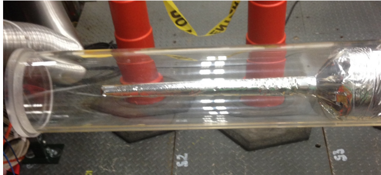
Figure 2.13: The liquid hydrogen target cell for the GlueX experiment. Beam enters from the right of the image.
