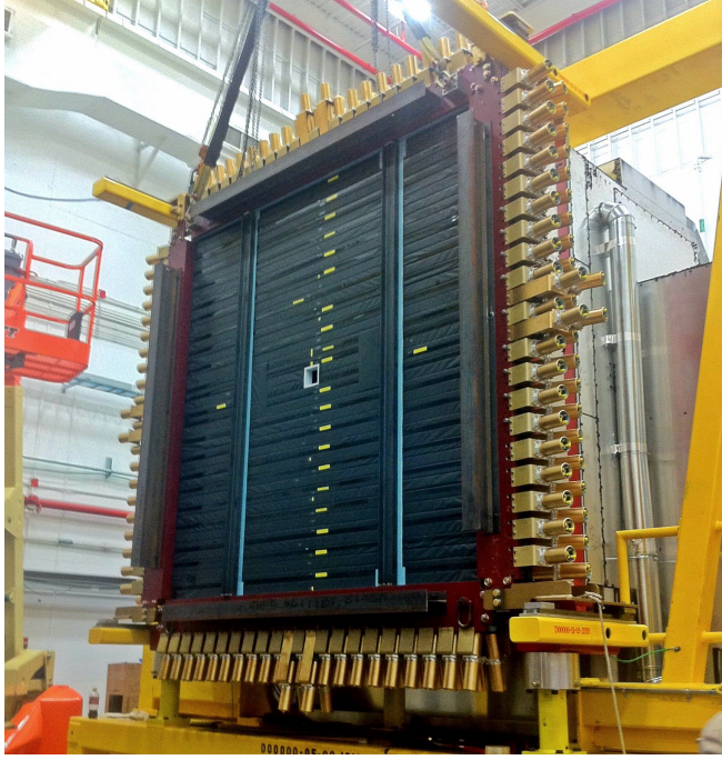
Figure 2.27: The TOF detector mounted on its support frame.
