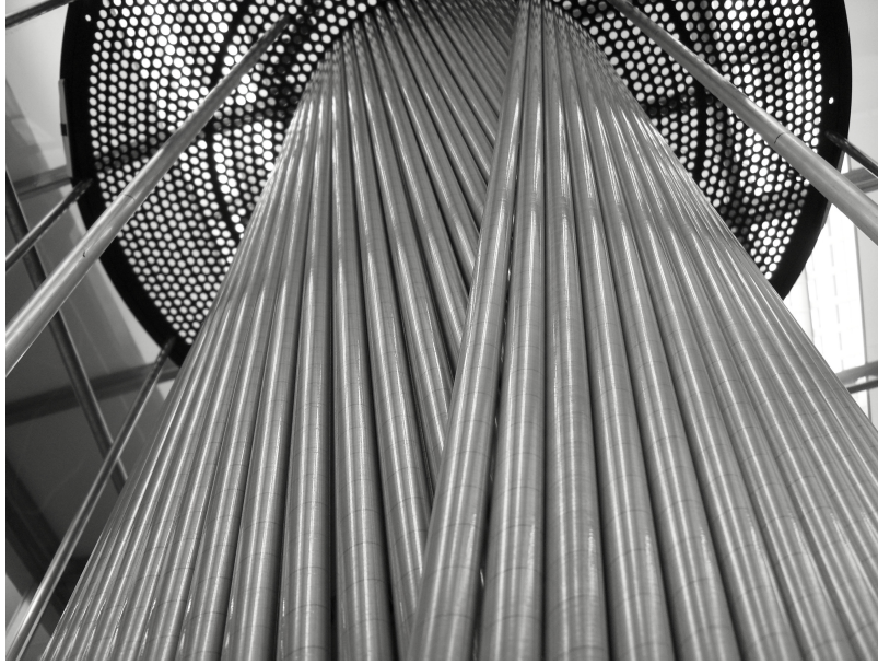
Figure 2.20: Picture showing two opposite stereo layers during construction of the CDC.
