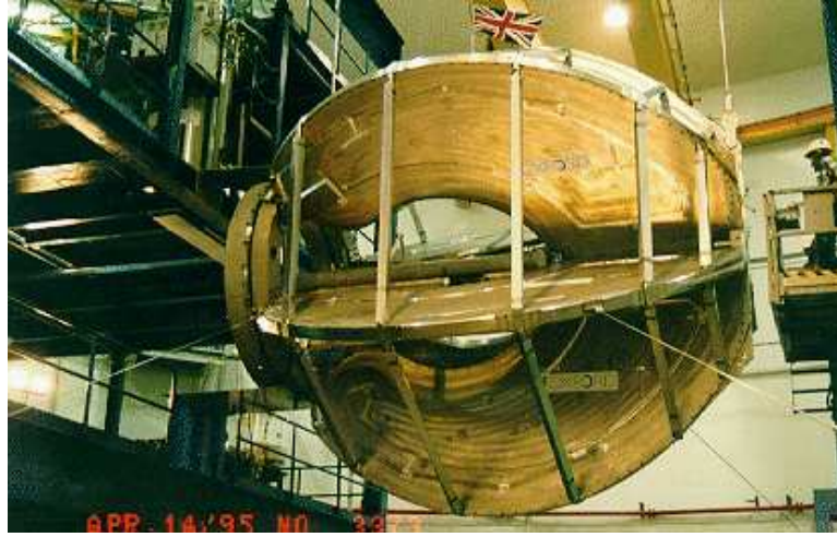
Figure 2.12: Photograph of the CLAS Superconducting Toroidal Magnet. Image source: [47].
