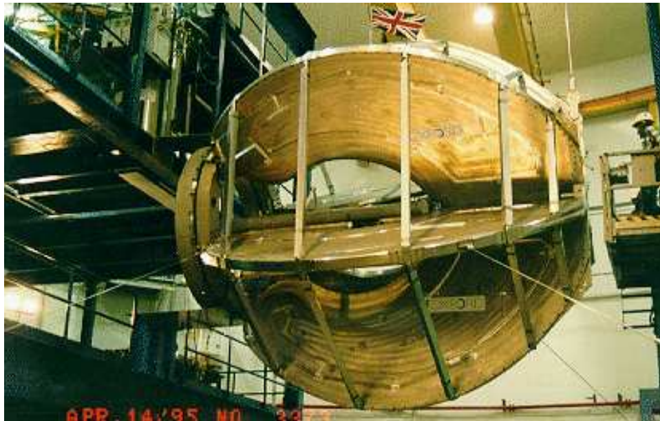
Figure 2.12: The bare coils for the CLAS toroidal magnet in place on the carriages that hold the detector. The cross members were actually thin carbon-fiber posts. Image source: [22].
