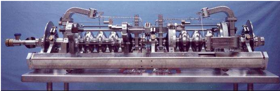
Figure 2.3: A pair of CEBAF's superconducting RF cavities, shown here with support hardware and beam pipe. Image source: Ref. [30].
