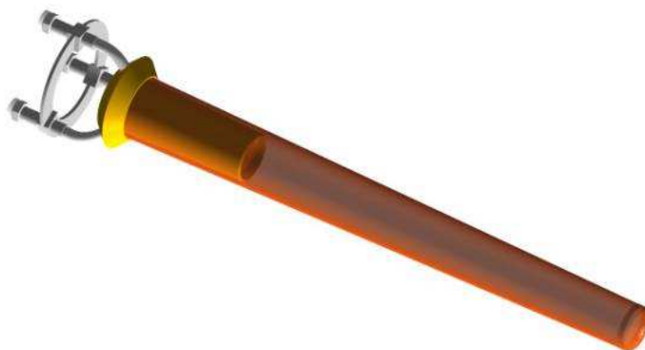
Figure 2.10: Target cell used during the g_{11a} run period. Image source: Ref. [39].
