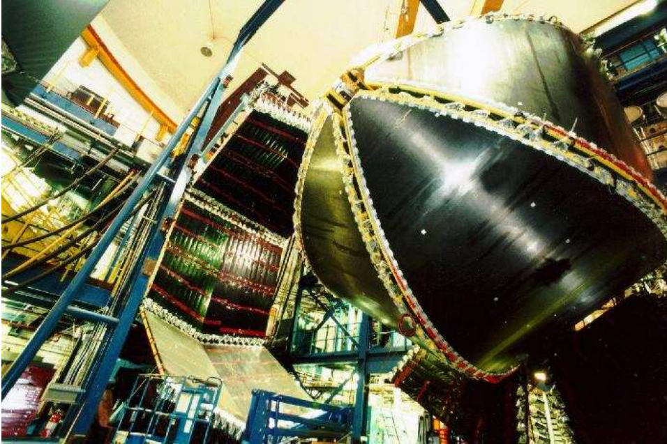
Figure 2.8: Photograph of the CLAS detector taken during a maintenance period for which the time-of-flight scintillator walls, forward region Cerenkov counters and electromagnetic calorimeters were pulled away from the interior detector elements. Image source: Ref. [30].
