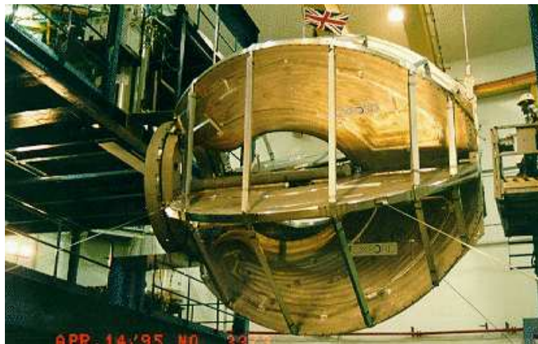
Figure 2.12: The coils of the CLAS toroidal magnet prior to installation of the rest of the detector subsystems. Image source: Ref. [30].
